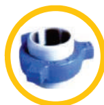
Fig. 200 Blue Nut Gray Subs A precision metal-to-metal sealing surface between male and female subs for air, water, oil, gas and mud service to 2,000 psi NSCWP*.
