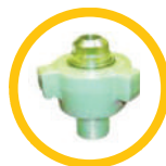
Fig. 2202 Green Nut Green Subs Especially for sour gas service; with heat-treated components, fluoroelastomer seal rings. For service to 15,000 psi NSCWP*.
