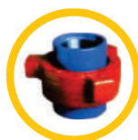
Fig. 1002 Red Nut Blue Subs A resilient lip-type seal protects ball and cone seal against abrasion in air, water, oil, gas and mud service to 10,000 psi NSCWP*.
