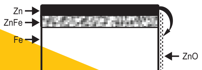
Protection of cut edges with zinc coatings.
