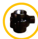
Fig. 400 Black Nut Red Subs Features a precision ball and cone sealing surface for sure metal-to metal seal for air, water, oil, gas and mud service to 4,000 psi NSCWP*.
